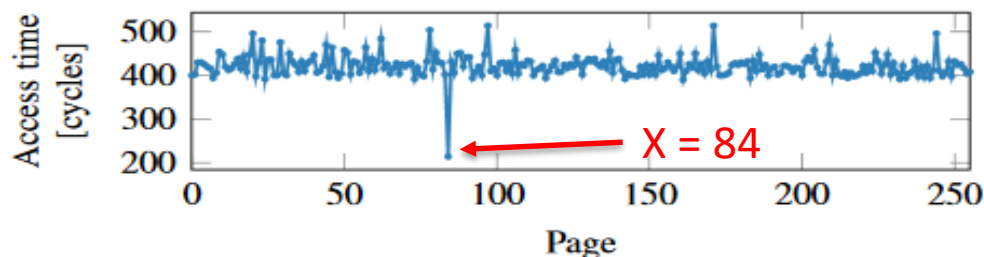
Figure 4: Even if a memory location is only accessed during out-of-order execution, it remains cached. Iterating over the 256 pages of probe_array shows one cache hit, exactly on the page that was accessed during the out-of-order execution.
