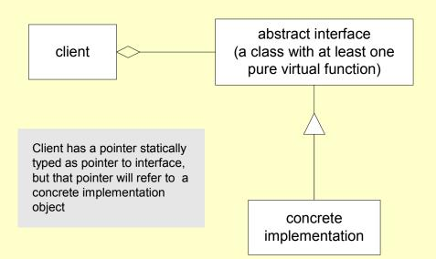
The purpose of an abstract interface is to provide a protocol for clients to use to request service from concrete objects without coupling to their implementations
